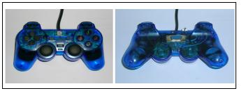
Figure 2. A Dualshock-like USB joystick (left) and a hacked joystick showing the nine-pin D-sub-miniature connector mounted underneath the controller and the analog joystick axis switch (right).
