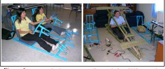
Figure 6. Racing game controllers made from PVC water-pipe (left) and bamboo (right).
